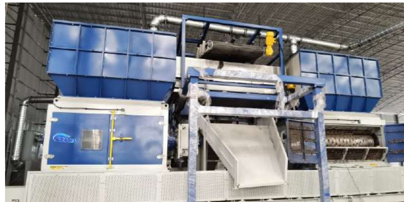
搭配撕碎机和输送带，可组成简易破碎线。 Integrating with shredder and conveyor to set up a shredding system.
