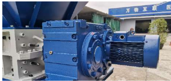
两台独立电机驱动加上高安全系数减速机产出超高扭矩。 2 independent drives with gear reducers bring a high torque.
