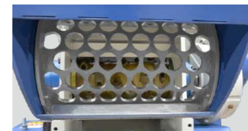
筛网 Screen 孔径可选，决定颗粒尺寸。 Customizable screen opening for granule size control.
