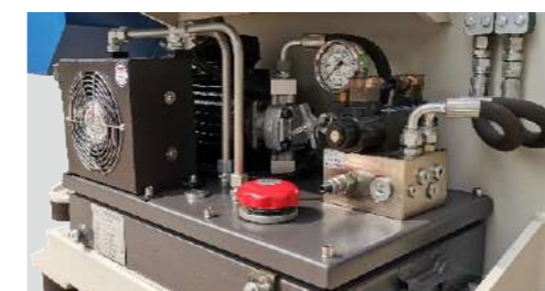
液压站 Hydraulic Station 推料箱的强力驱动，物料更好贴合刀辊。 Powerful drive to pusher ram against rotor.
